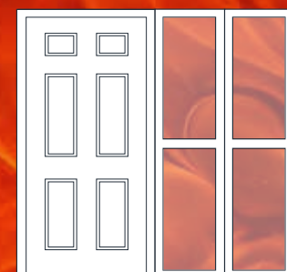
Coupled glazed doubled side screens
